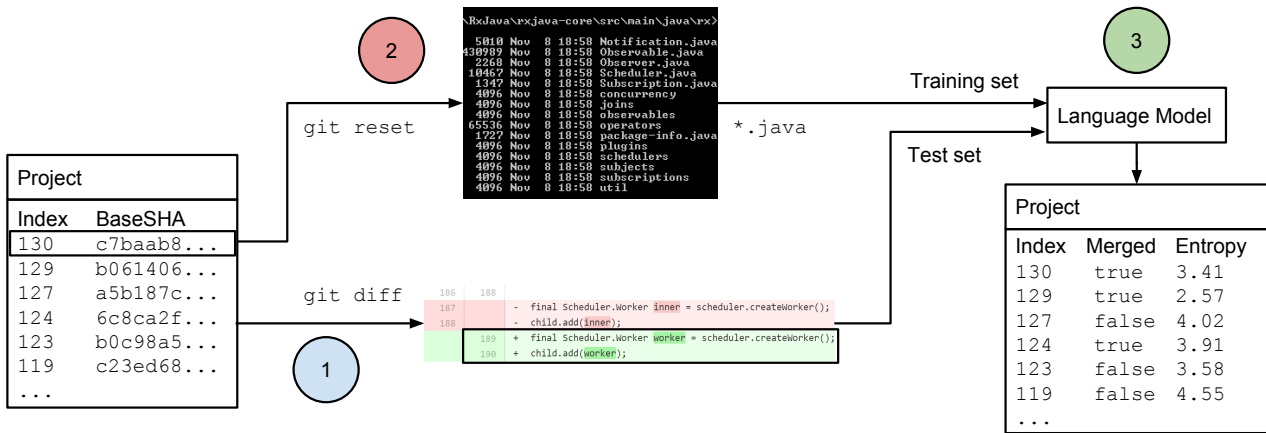
Figure 2. An overview of the setup used to acquire entropy scores for pull requests.
